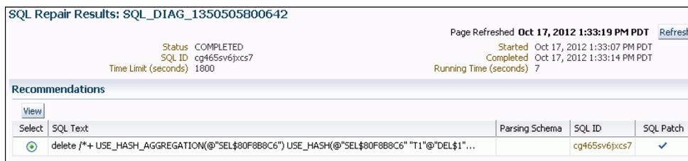
A check mark in the SQL Patch column indicates that a recommendation is present. The absence of a check mark in this column means that the SQL Repair Advisor was unable to devise a patch for the SQL statement.
